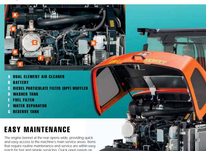
reach for fast and simple servicing. Quick-open panels on the right and left sides provide speedy access to the fuel refill (right side) and battery (left side). Other areas of the R070 and R090 are also easy to service and maintain.
